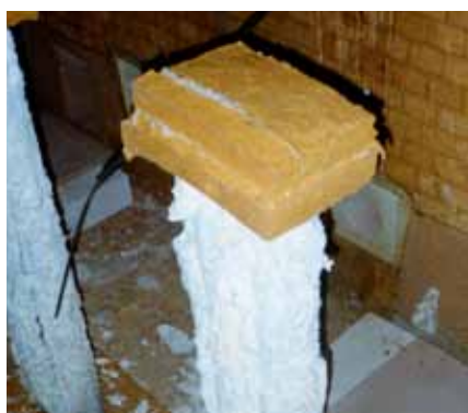
Brandwerende coating na verhitting
